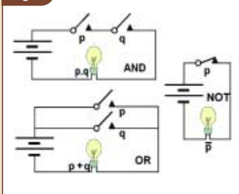
Similarly in an 'OR' circuit the lamp will light if either (or both) of its relays is shut, corresponding to the truth table at fig.4. In the 'NOT' circuit, relay p is fitted with a 'break', rather than a 'make' contact. The lamp is therefore lit (true) when the relay is open (false), and is extinguished (false) when the relay is shut (true - see fig.5). The analogy is rather like a succession of gates opening and shutting.
